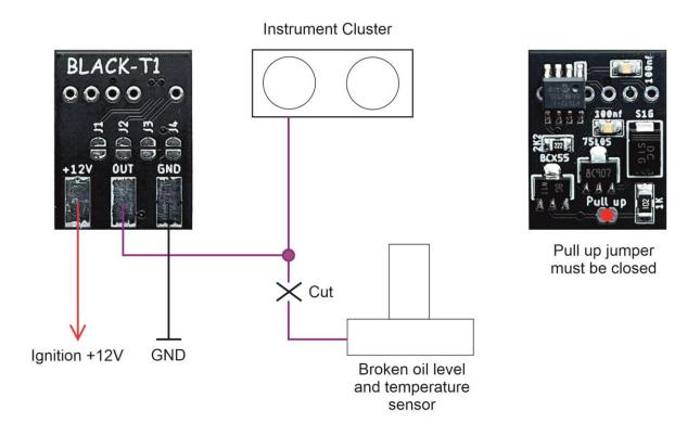
[!] MB/ Volvo Oil level sensor connected to engine ECU, not to instrument cluster.
