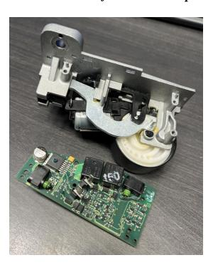
**NOTE:** PCB of ESL can be two types: With ELMOS or with Motorola MCU. Examples in photo below. ESL emulator works with both types of PCB.
